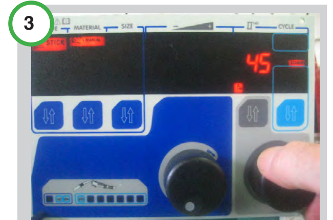
3 ADJUST THE WELDING DYNAMIC: With the second knob, adjust the desired value The dynamic can be adjusted from 0 to 100% Dynamic increase the current for arc striking Dynamic increase the current during drop transfer.
