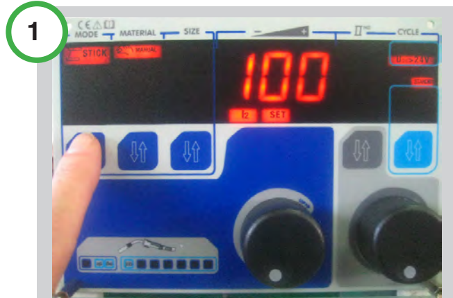
1 GB SELECT MMA IN MANUAL: With the first push button, select STICK With the second push button select MANUAL With the main knob, adjust the welding current.
