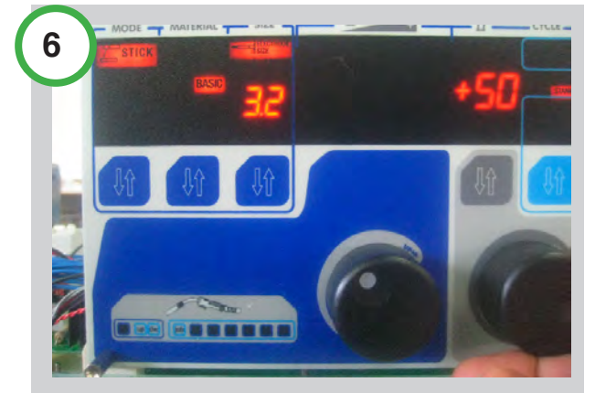
6 ADJUST THE WELDING CURRENT AND DYNAMIC: With the FIRST knob, adjust the desired value, the second display shows the material thickness. Dynamic is automatic, but can be increased or Decreased in % as the operator desire.
