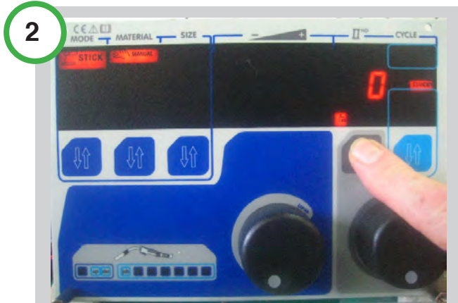
2 ADJUST THE WELDING DYNAMIC: With the forth pushbutton select the dynamic icon. The second display show the current set value.
