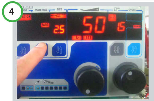
4 SELECT MMA IN SYNERGYC: With the second push button, select the type of the electrode.
