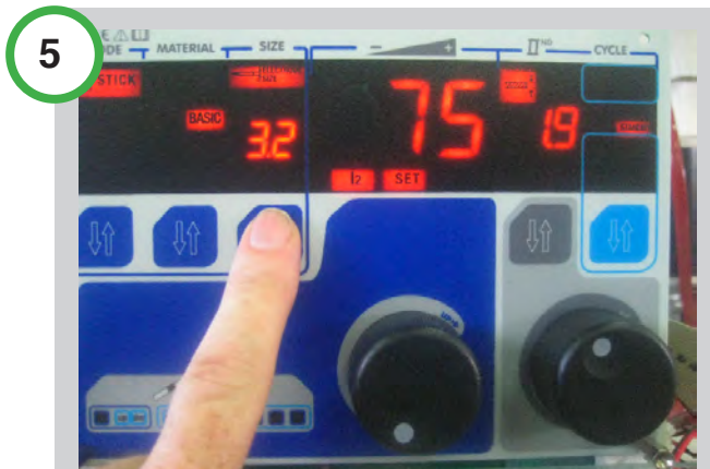
5 SELECT MMA IN SYNERGYC: With the third pushbutton select the size of the electrode.
